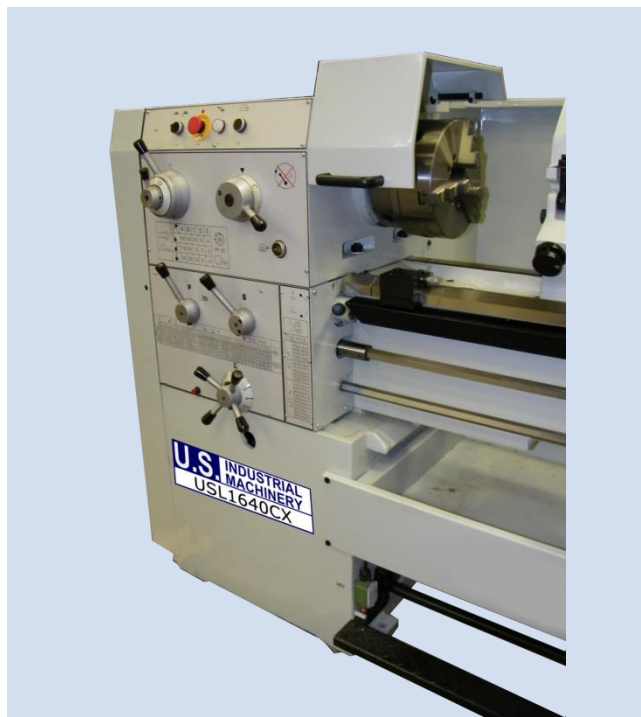
Detail of Headstock, chuck and guard
