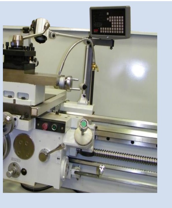
Detail of Apron, 4-way rapid, digital readout.
