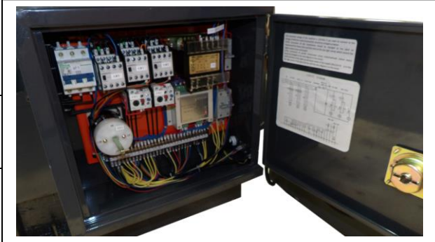
Detail showing control panel with reciprocation and electric motor table crossfeed control selection.
