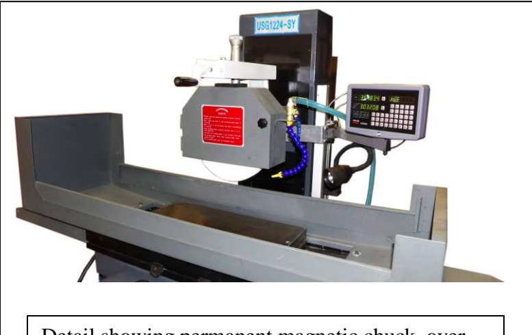
Detail showing permanent magnetic chuck, over wheel diamond dresser, 2-axis digital readout display, flood coolant nozzle
