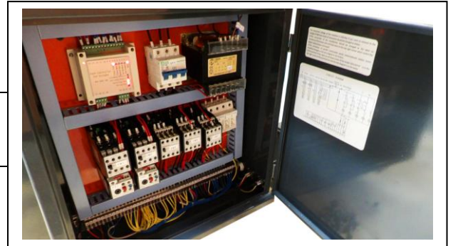
Detail showing control panel with reciprocation and electric motor table crossfeed control selection. Also with motorized wheelhead elevation.
