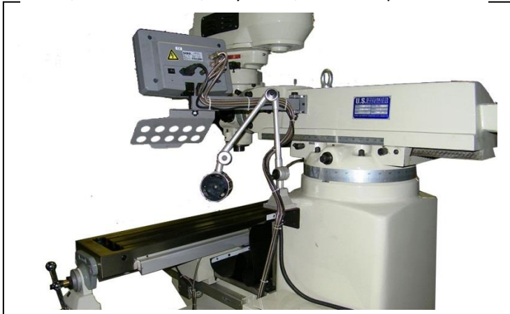
Detail of work light, digital readout, collet rack, table feed, coolant nozzle, way cover, ram and spindle
