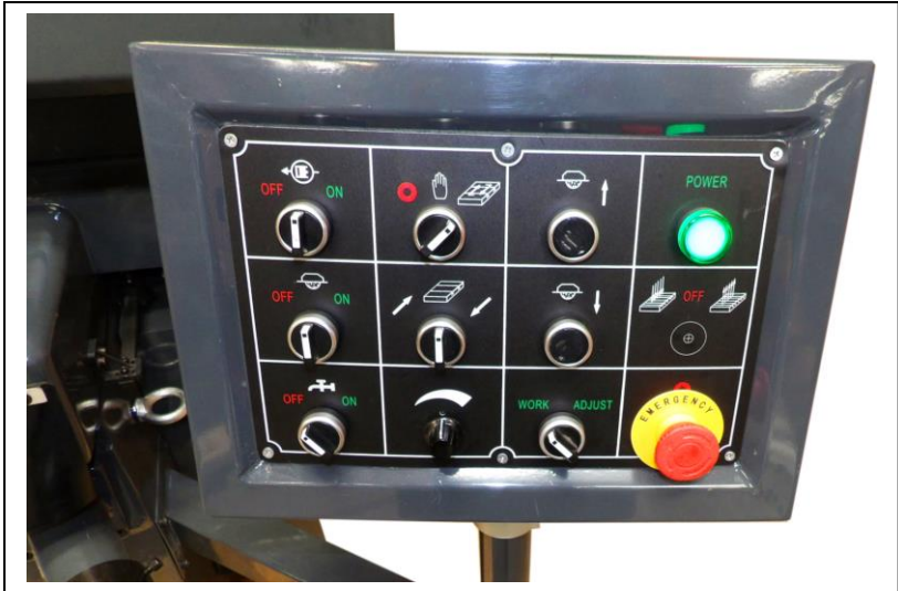
Detail showing control panel with reciprocation and electric motor table crossfeed control selection. Also with motorized wheelhead elevation.
