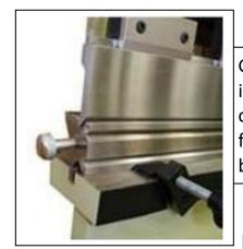
Gooseneck Punch Tool Sections included, full length of Ram. Multi-opening V-Die for up to 90 degree forming included, full length of bed. Die lifting rings included.
