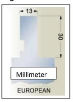
Our **bed** has slot for the Standard Die Tang as shown below. Also, bed tooling without tang can be held with the included capture clamps.
