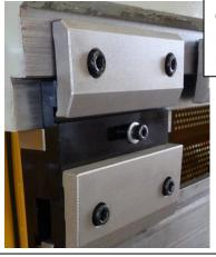
Our **optional** ram clamps for all punch Tangs shown above. Lever action allows for quick tool change.
