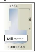
Our **bed** has slot for the Standard Die Tang as shown below. Also, bed tooling without tang can be held with the included capture clamps.
