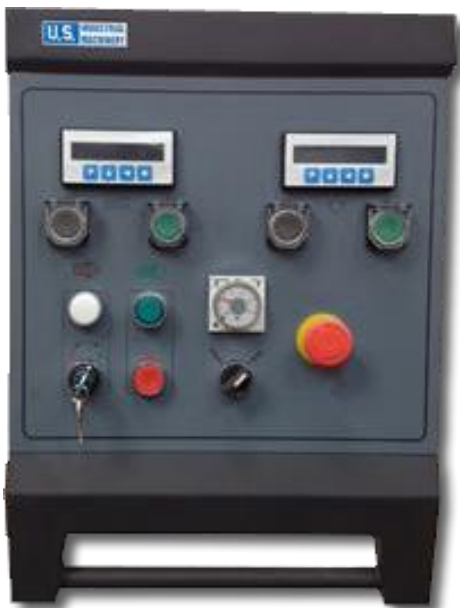
Photos above are manual Hydraulic Press Brake with front-operated power backgauge, power ram adjustment, both with manual fine adjustment and digital readouts. Operator's pendant has dwell adjustment for ram, key lockout, jog control and E-stop.
