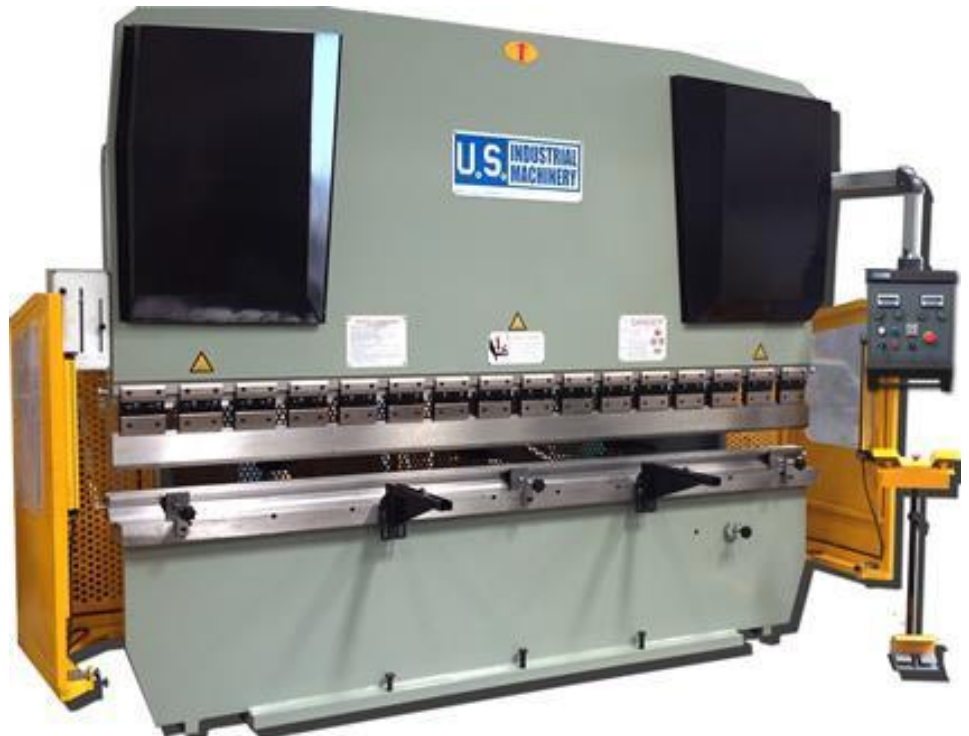
Photos above are manual Hydraulic Press Brake with front-operated power backgauge, power ram adjustment, both with manual fine adjustment and digital readouts. Operator's pendant has dwell adjustment for ram, key lockout, jog control and E-stop.
