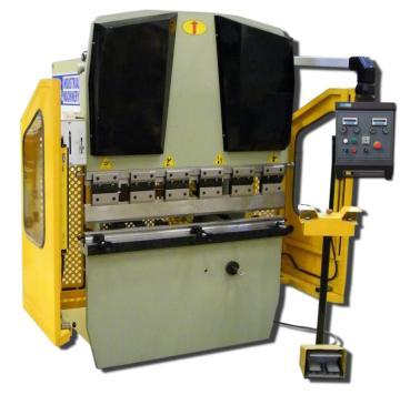
Photos above are manual Hydraulic Press Brake with front-operated power backgauge, power ram adjustment, both with manual fine adjustment and digital readouts. Operator's pendant has dwell adjustment for ram, key lockout, jog control and E-stop.
