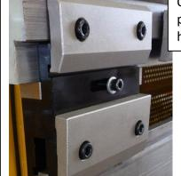
Our **optional** ram clamps for all punch Tangs shown above. Lever action allows for quick tool change.
