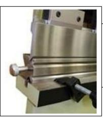
Gooseneck Punch Tool Sections included, full length of Ram. Multiopening V-Die for up to 90 degree forming included, full length of bed. Die lifting rings included.
